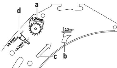
**a** The saw blade must be no more than 254 mm in diameter.
